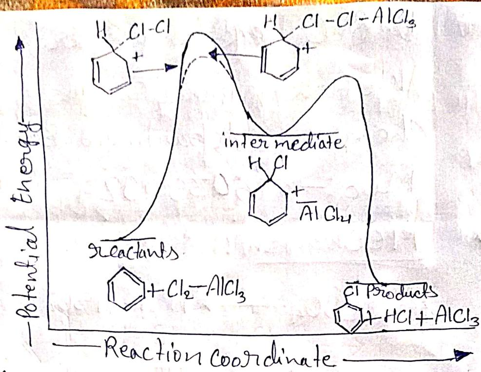
Schematic potential energy diagram for the chlorination of benzene with  $\text{Cl}_2$  and  $\text{Cl}_2\text{-AlCl}_3$  as the electrophile.
